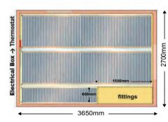
From these sizes we can calculate that we require 2 pieces of 3.5m length and 1 piece at 2m.
