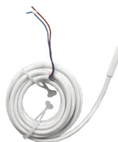
External sensor NTC type 10k \Omega at 25°C ( \beta = 3950 )
